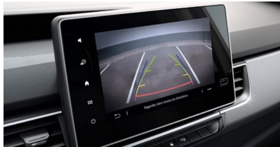
rear-view camera. It provides a rearward view on the easy link screen or the interior rear-view mirror when you engage reverse gear. Superimposed outlines make your manoeuvres easier and safer.
