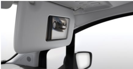
wide view mirror. Located in the passenger sun visor, it improves your vision and helps to minimise the effect of blind spots at Y-junctions. Available as standard on Advance models.
