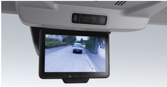
rear view assist. Via a digital screen – instead of the interior rear-view mirror – you can view what the camera installed at the rear of your vehicle sees.
